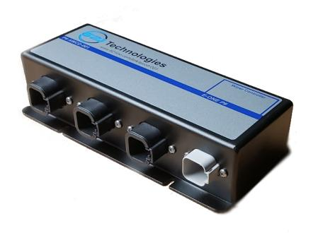
Advanced wiper controller includes delays, intermittent wipers and multiple wiper synchronization.
