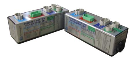
The device is designed for mobile applications and features robust packing, wide temperature and voltage tolerance as well as strong EMI and ESD immunity.
