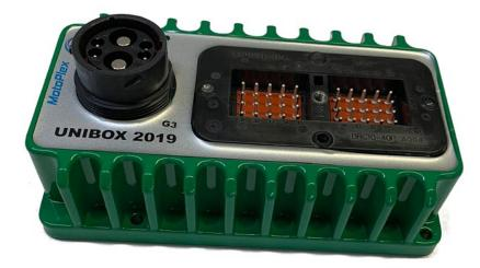
The device is designed for mobile applications and features robust packing, wide temperature and voltage tolerance as well as strong EMI and ESD immunity.
