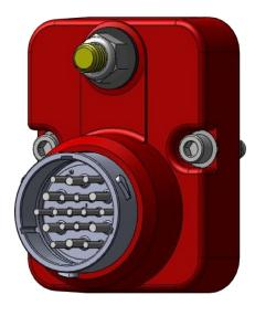
This device is a corrosion proof alternative to the typical ring terminals on a stud approach often found in heavy vehicle and marine applications. The 300 Amp stud is connected to a fully encapsulated solid copper bar tied in parallel to all connector terminals. The industry standard Deutsch connector provides a robust time tested mass termination point.
