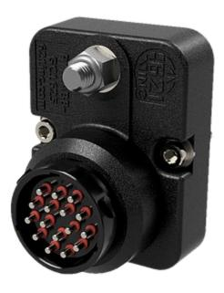
This device is a corrosion proof alternative to the typical ring terminals on a stud approach often found in heavy vehicle and marine applications. The 300 Amp stud is connected to a fully encapsulated solid copper bar tied in parallel to all connector terminals. The industry standard Deutsch connector provides a robust time tested mass termination point.
